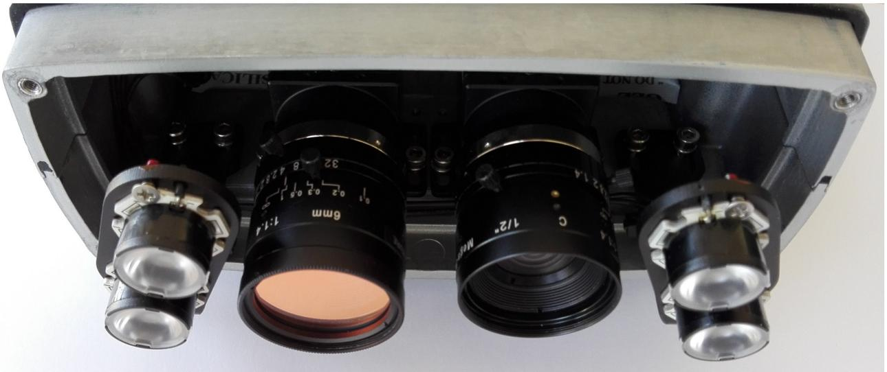
Each lens has two rings. The ring closer to the camera's sensor is the IRIS, while the other controls the focus. If you wish to refocus the camera, loosen the knob and re-adjust the focus. When the operation is completed do not forget to retighten the knob.
